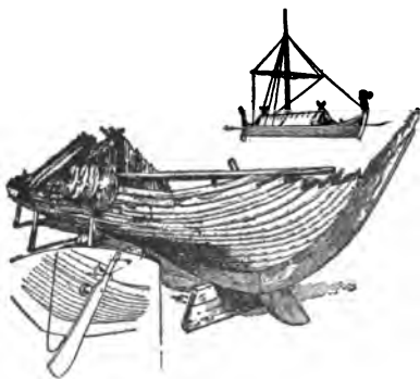
THE BOW OF THE VIKING SHIP OF GOKSTAD, SHOWING RESTORED STEERING BOARD ON THE LEFT, AND COMPLETE SHIP ABOVE
